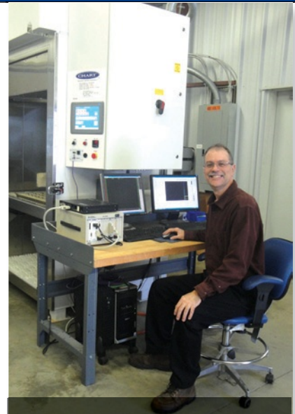
Gary Delserro sits at his lab's Highly Accelerated Life Test (HALT) Chamber, which performs combined temperature and vibration loads simultaneously.
